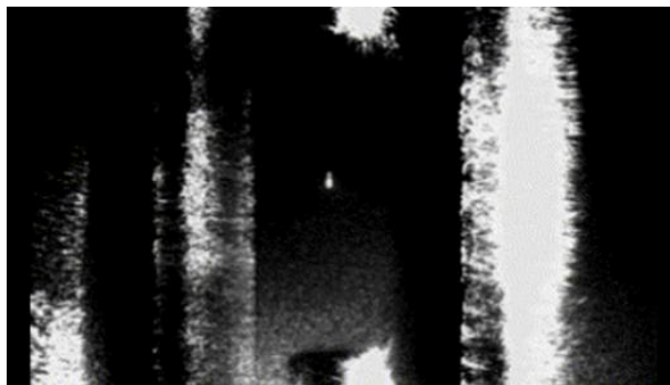
Figure 1.3: Image illustrating the charged nanoparticle (the white dot near the center of the image) trapped in the Paul trap used for the first experimental proof of concept. On the center-top and center-bottom the endcaps can be seen, illuminated by the laser and at about 1 cm from each other, while the vertical bars on the side are the RF electrodes. The direction of the gravitational acceleration is the same of the Paul trap axis, and is pointing downwards.
